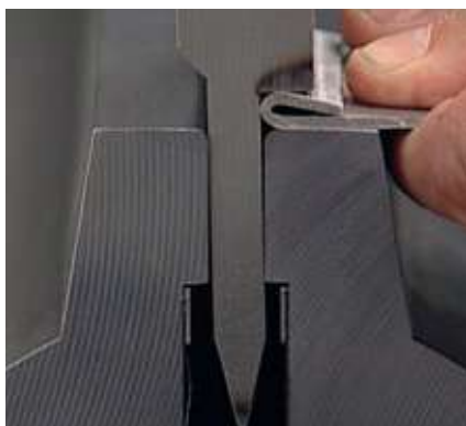
Pre-bend and flattening in the same tool.
